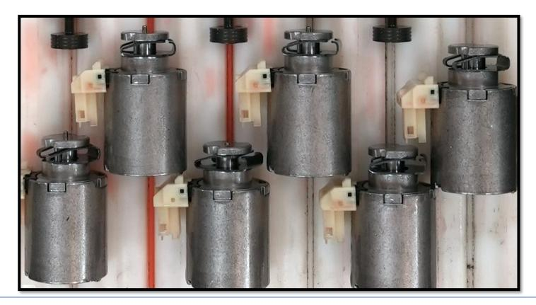
Linear Solenoids use a mechanical pintle to push on the hydraulic valve. Nothing new, Toyota and Honda has been doing this for a while. The 10R/L doesn't use springs to return the valve/pintle. Backfill pressure is used to return
