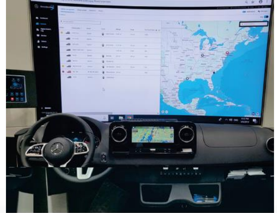
GPS data supplies the vehicle map. Location is tracked by a telematics service provider.
