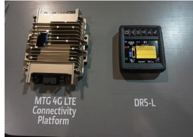
A cell phone module that connects the CAN to a mobile telematics network.
