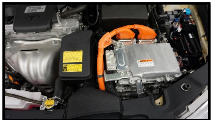
Toyota hybrids packages their DC-DC converter with the inverter electronics. They share the same cooling system.
