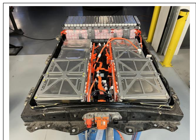
High voltage battery from a 2016 Nissan Leaf
