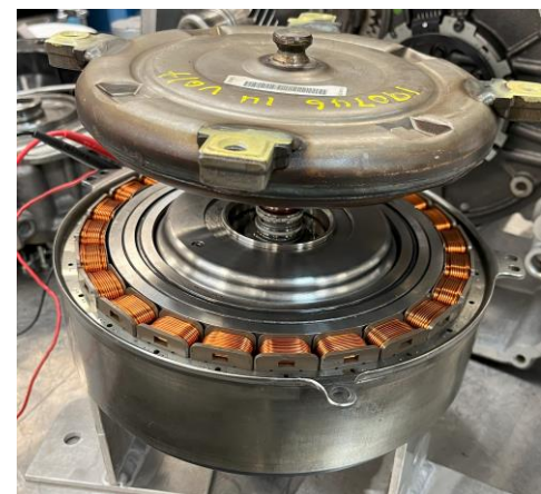
High voltage motor with the torque converter from a Ford F150 Hybrid
