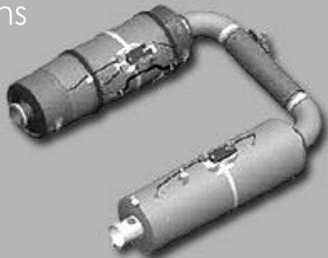
Horizontal DPF - Horizontal SCR, Frame Rail Mounted
