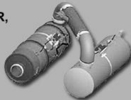
Horizontal DPF - Horizontal SCR, Frame Rail Mounted
